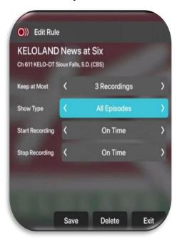
Scroll through the list and highlight a series that you want to manage. Press the center of your remote to open an Edit Rule screen.
